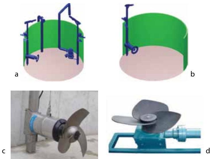
Figure 10.14 Mechanical manure mixers [2, 5]
